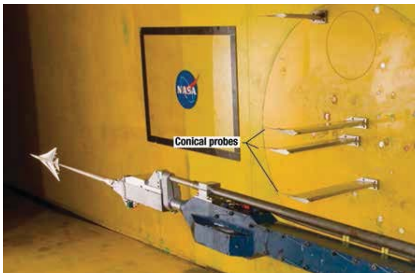
(a) Conical (2° half-angle cone) probe measurements (on- and off-track).
