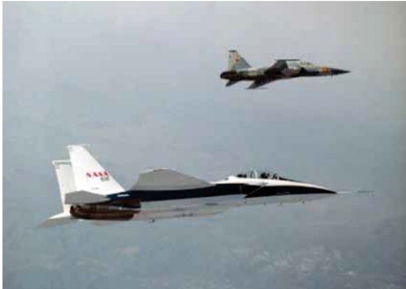
Figure 4.16. An instrumented NASA F-15B aircraft probes an F-5E supersonic flow field on an Inlet Spillage Shock Measurements (ISSM) flight test high above the Mojave Desert at Edwards Air Force Base, California in 2002.
