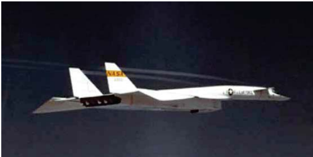
Figure 4.9. During the 1966-67 U. S. National Sonic Boom Program, sonic boom signatures were acquired above and below the XB-70, which was flown at an altitude of about 37,000 feet, a speed of Mach 1.5, and a weight of about 333,000 pounds.
