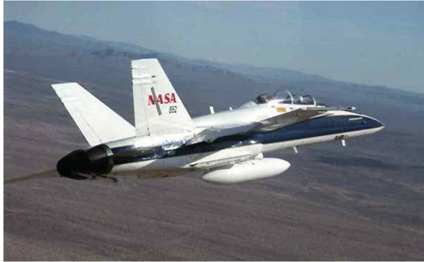
Figure 8.23. In June 2006 and July 2007, NASA conducted low sonic boom flight tests of an F/A-18B Hornet at the NASA Dryden Flight Research Center (DFRC) in California.
