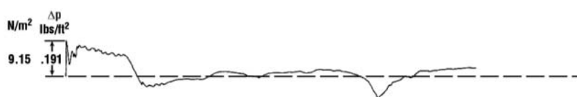
(b) Measured on USS Austin , Overhead Conditions: Velocity = 4762 m/sec and Altitude = 178,778 meters.
