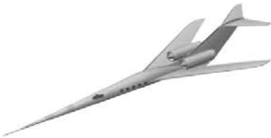
(a) High-speed concept with deployed quiet spike.
