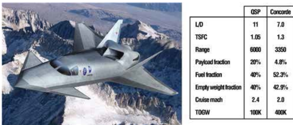
Figure 7.92. Quiet supersonic platform concept and design goals (ref. 7.65).
