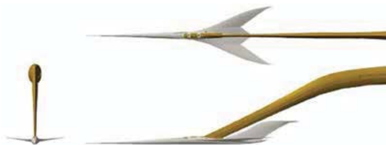
(a) Three-view drawing of wing-body-vertical low-boom aircraft concept with a blade mount.
