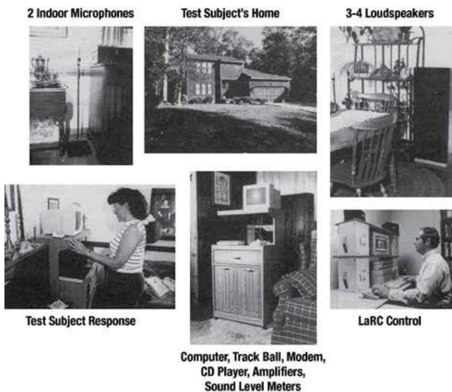
Figure 9.127. In-home noise generation/response system (ref. 9.76).
