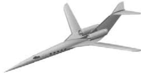
(b) Low-speed concept with stowed quiet spike.
